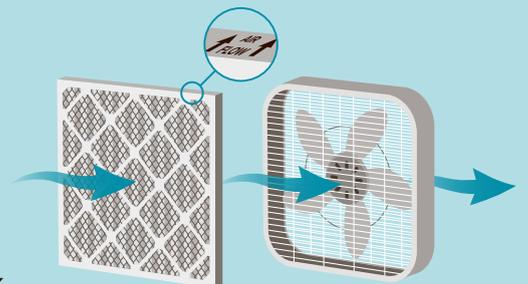
**Attach filter to back of fan with bungee cord or tape.**
